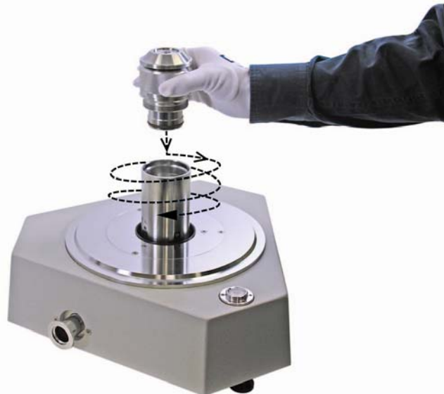
Figure 4. Piston-Cylinder Module Installation
