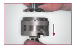
Step 1: Retract Collar Slide collar to open position. This opens the connector locking assembly.
