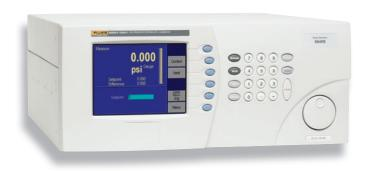
The 7250LP low pressure controller/calibrator, part of the versatile Series 7250 family, is specifically designed to meet the demanding performance requirements of calibrating low pressure sensors, transducers, mechanical gauges, portable calibrators and their plug-in modules. To accommodate bidirectional devices, the 7250LP can be supplied to operate in both positive and negative gauge modes.
