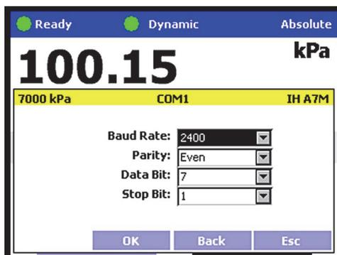
A field, such as **Baud Rate**, **Parity**, **Data Bit** or **Stop Bit** in the COM1 screen is in drop down menu format. *Enter* one of these fields to display a list of the selections available.
