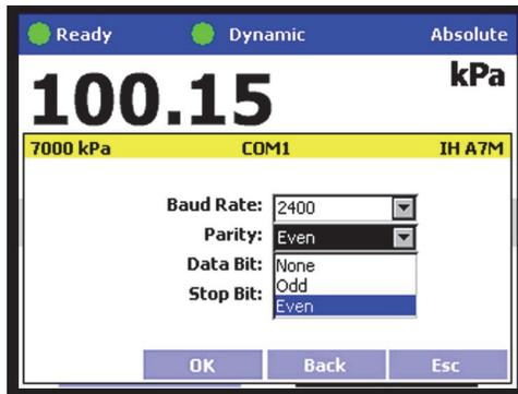
Continuing Example 5, entering **Parity** displays a list. *Select* and *Enter* to accept the new parity value.
