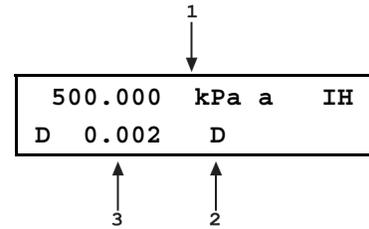
Observe the *Ready/Not Ready* indicator LED (see Section 3.2.3) for indication of when the controlled pressure has reached the target and stabilized. PPC4 continues controlling following static or dynamic control operation protocol (see Section 3.2.2) until automated pressure control is interrupted.
