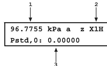
*Enter* the value of the AutoZ reference ( $P_{std,0}$ ) in the same unit of measure as the top line display and **ENTER**. PPC4 logs the readings and calculates a new AutoZ offset value. The next display is:
