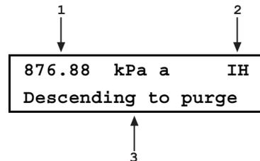
PPC4 controls pressure down to less than 700 kPa (100 psi), stops control and displays **<Preparing to purge>** for five seconds. After the five second delay, PPC4 opens the SPLT exhaust valve and displays **<PURGING>**.
