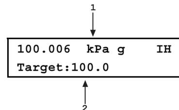
Edit the target pressure value as desired (see Section 0 for information on zero pressure commands).
