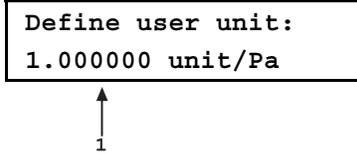
Enter the number of user units per Pascal (Pa) in the entry field. **ENTER** defines the user unit and returns to the **<Set up unit #n>** screen.
