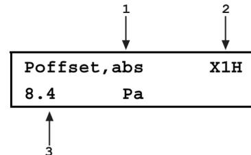
Edit  $P_{offset}$  as desired and **ENTER** to activate the new value. **ESC** to abandon changes.
