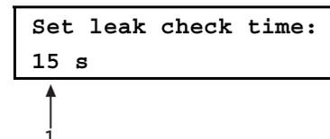
Edit the leak check time if desired (minimum 1, maximum 999) then **ENTER**. **ENTER** again when ready to start the leak test. The leak test display is:
