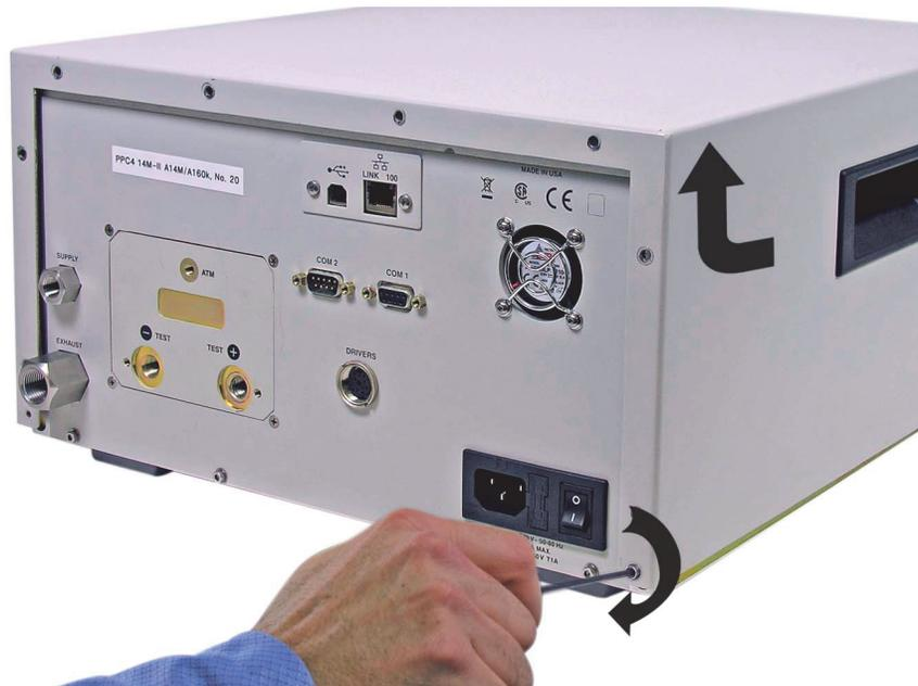
**Figure 29.** Removing Back Cover
