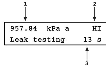
**ESC** can be used to abort the running leak test. **ENTER** while the leak test is running restarts the leak check timer. When the leak check timer countdown has completed, the leak check results screen is displayed:
