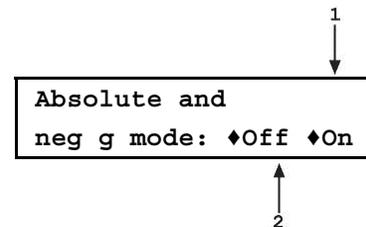
If in **edit** mode, the OFF or ON status can be changed by selecting **<Off>** or **<On>** (see Section 7.2.5). **ENTER** in view mode returns to the view/edit screen. **ENTER** in edit mode goes to confirmation of change activation if changes have been made. **ESC** from any edit screen exits the edit screen without activating any changes.
