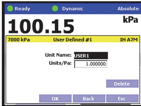
To create or edit a User defined unit, *Enter <User units>* in the Unit screen. *Enter Units/Pa* and input a value using the numeric key pad.
