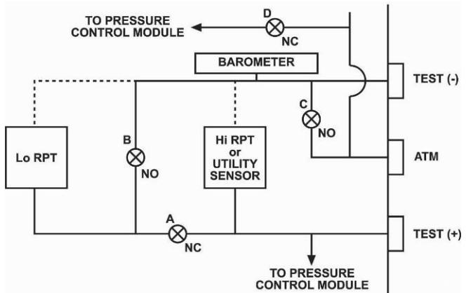
**Figure 32.** Q-RPT Module Schematics for Various Configurations
