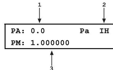
If in **edit** mode, the calibration fields can be edited. If the selected Q-RPT is an Axxx Q-RPT, pressing **ENTER** in the **PM** field continues to the next calibration information display (this display is skipped if the Q-RPT is an Gxxx or BGxxx):
