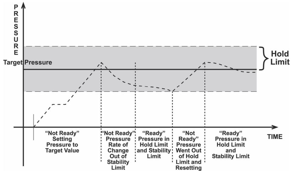
Figure 7. Ready/Not Ready in Static Control Mode
