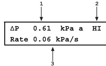
From the leak check results screen, **ENTER** to repeat the leak test.
