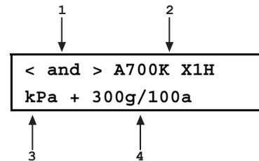
Use the cursor control keys to toggle through the ranges available to be deleted. When the desired range to be deleted is displayed, **ENTER**. If you are sure you want to delete this range, **ENTER** again in response to the **<Delete?>** query. **ESC** to return to the AutoRange screen without deleting a range.
