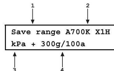
**ENTER** to save the range or **ESC** to return to the Main Run Screen without saving the range.
