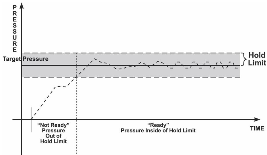
Figure 6. Ready/Not Ready in Dynamic Pressure Control Mode
