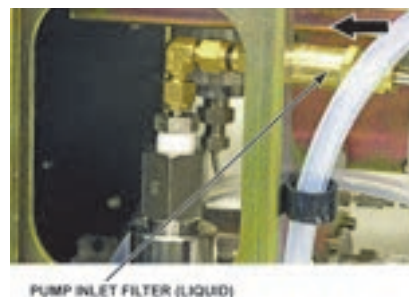
Previous Pump Supply Filter P/N 3068879 (103727)
