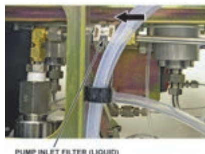
New Pump Supply Filter P/N 3138000 (102808)
