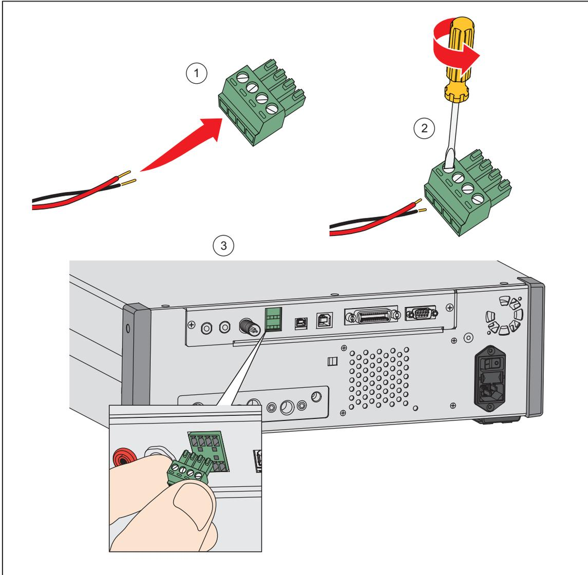
Figure 20. Driver Connections
