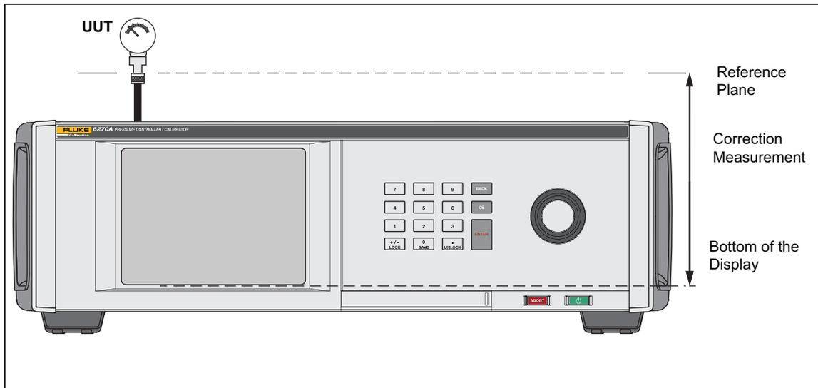
Figure 8. Head-Height Correction
