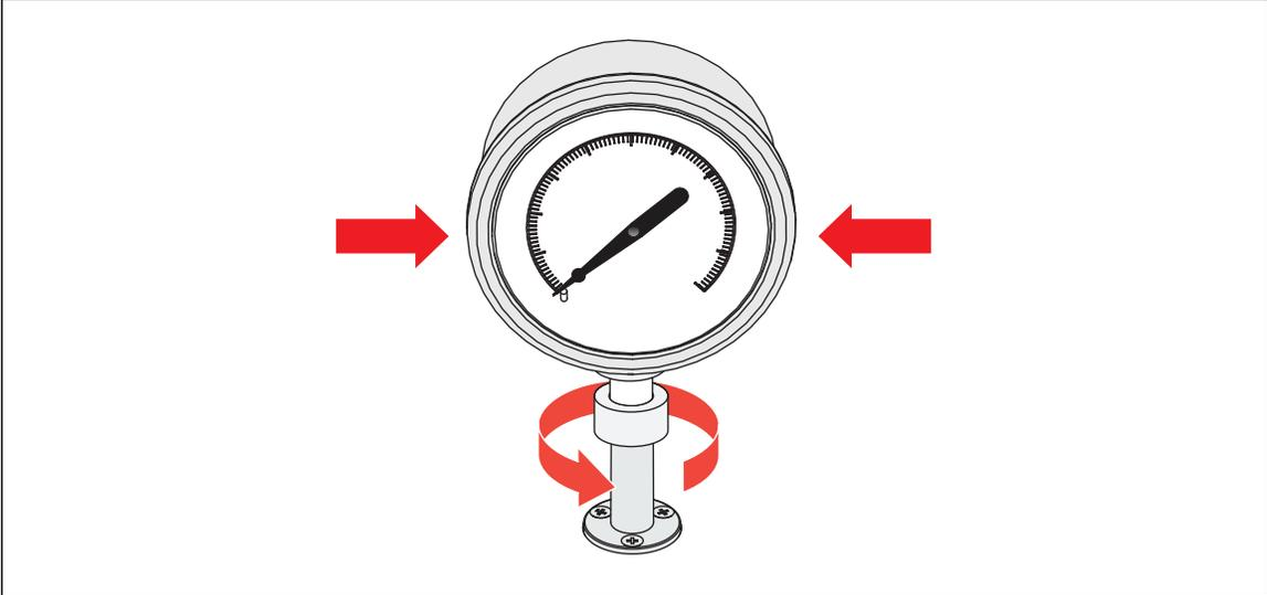
Figure 14. Tighten Gauge
