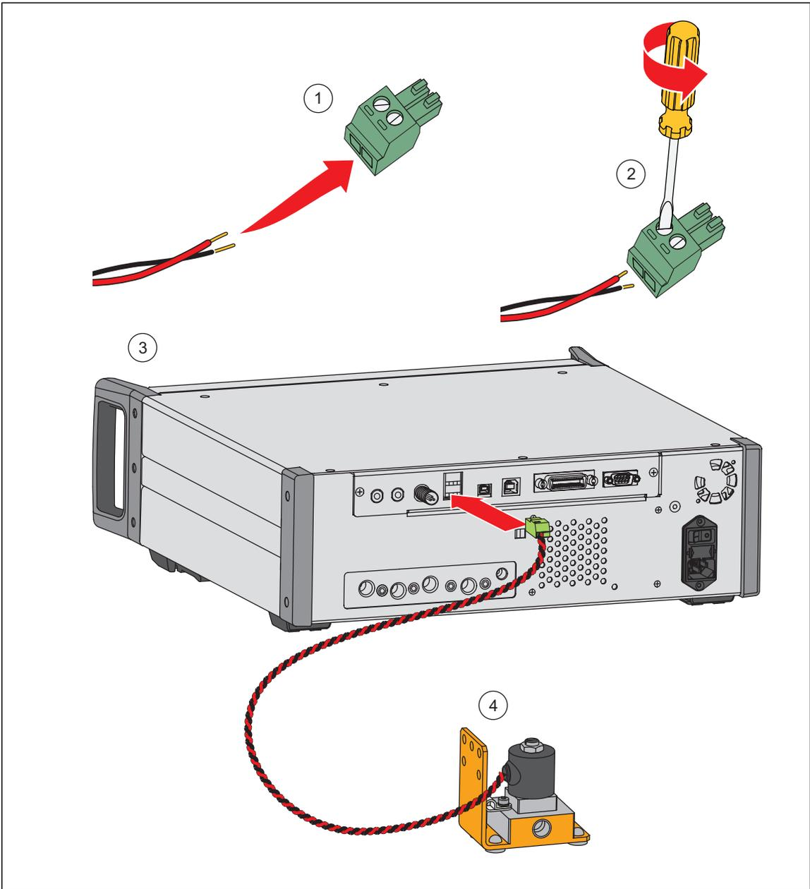
Figure 21. External Isolation Valve Connection
