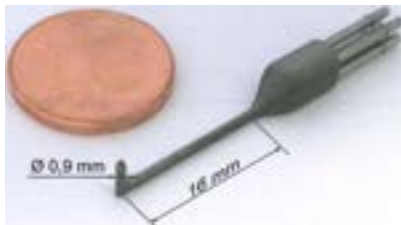
Miniature Probe. Head \Phi 0.9\text{mm}
