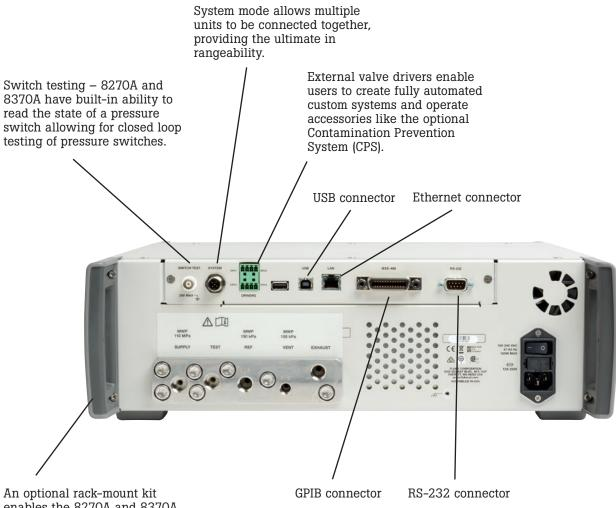
An optional rack-mount kit enables the 8270A and 8370A to be installed in a standard 19-inch rack.
