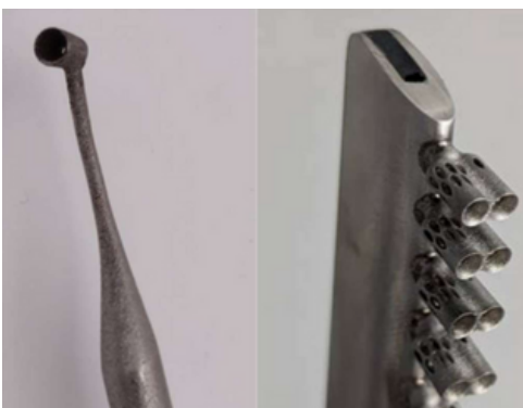
Fig. 1 Kiel probe (left side) and rake with several Kiel probe heads installed (right side)
