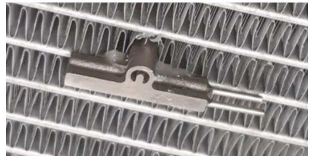
Fig. 4 Probe (S_KPS_bujh36) mounted on radiator from behind
