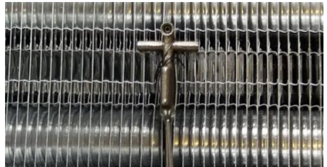
Fig. 3 Frontal mount of probe (S_KPS_qxpj) on radiator
