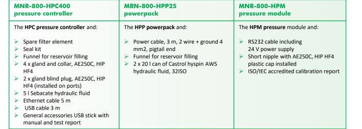
HPC system components standard delivery
