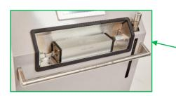
Interchangeable pressure modules HPC reference pressure modules are interchanged in minutes (see p. 5). This allows optimization of the pressure measurement range to the device under test range. The modules are compact, standalone, plug and play devices that can be calibrated independently of the HPC so the HPC does not need to be taken out of operation or moved for recalibration.
