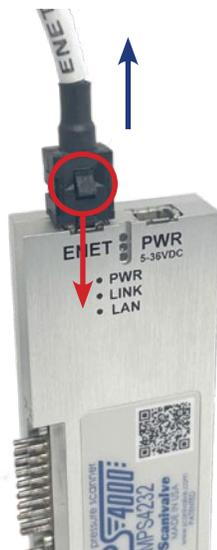
**FIGURE 4-4: POWER/ETHERNET CONNECTOR LATCH**
