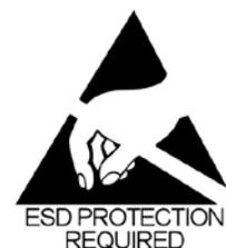
The ESD note symbol indicates that proper precautions for handling Electrostatic Sensitive Devices need to be taken when performing the related operation. This includes the use of grounded work surfaces and personal wrist straps to prevent damage to sensitive electronic components.
