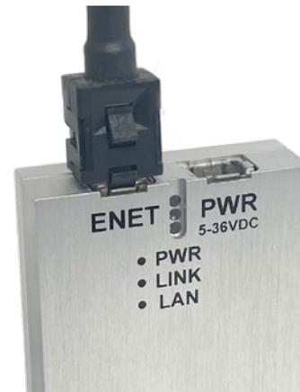
**FIGURE 2-3: POWER & ETHERNET CONNECTIONS**
