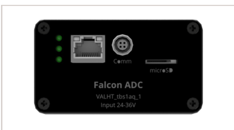
Fig. 2 Falcon ADC – Front view with connectors
