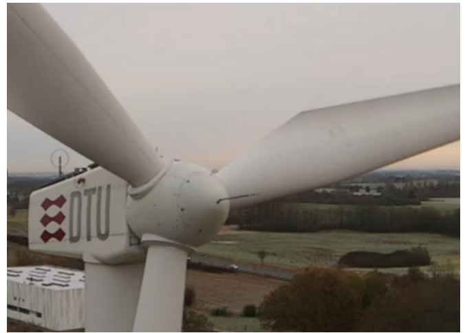
Fig. 3 Test turbine at DTU with Windflower system installed on the nose cone
