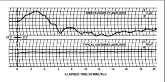
FIG. 2 EFFECT OF ABRUPT TEMPERATURE CHANGE
