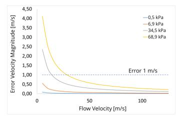
Figure 1: Dependence of velocity measurement error on pressure scanner range (0.05% FS accuracy)
