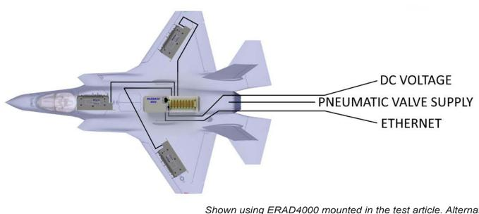
Shown using ERAD4000 mounted in the test article. Alternate system configuration uses DSM4000 installed under the test section or in the control room.
