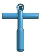
The Vectoflow radiator probes offer an easy way to equip a radiator with probes in order to measure total mass flow and mass flow distribution through a radiator. The radiator probe simultaneously measures the total and static pressure of the flow. Several probes distributed over a radiator can measure the partial mass flow through the assigned section of the radiator, allowing to determine the uniformity of the flow.
