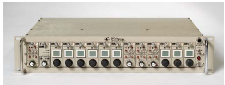
Model R408-14 Enclosure (rear view below)
