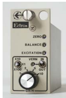
Model 352 Transducer Conditioner-amplifier
